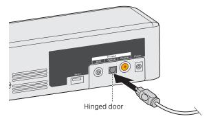
**Note:** The connector has a hinged door that swings inward when inserting the plug.
